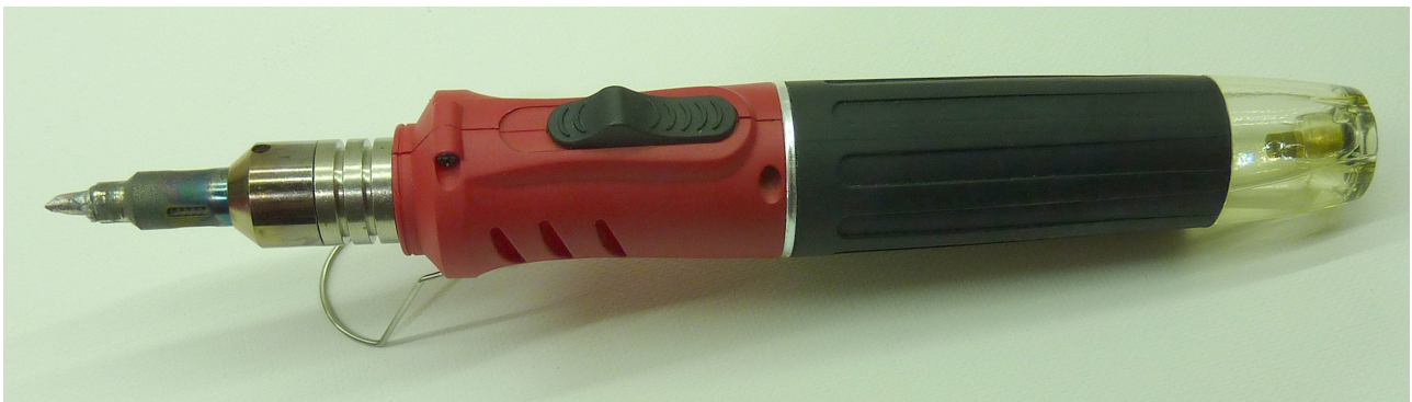
Gas soldering iron (no, not gasoline!) Photo Peter Scott
